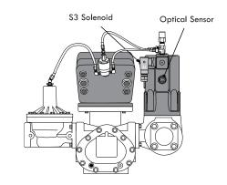
Meter System with Optical Vapor Eliminator
