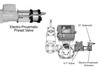
Single Stage Electro-Pnuematic Valve with V-7 Valve
