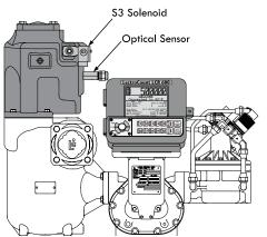
Meter System with Optical Air Eliminator
