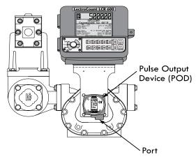
Meter System with Pulse Output Device
