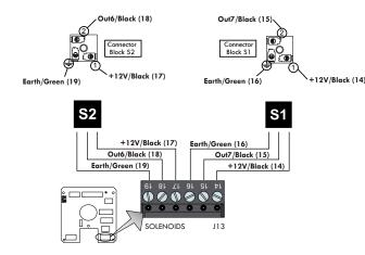
Solenoid 1 and Solenoid 2 Wiring for A2859-11 and 3-Way Two Stage, 2848-11 Two Stage, and E-7 Two Stage
