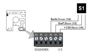
Solenoid 1 Wiring for Single Stage Valves
